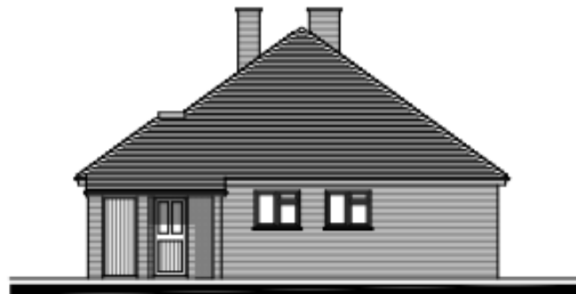
EXISTING NORTH EAST ELEVATION
